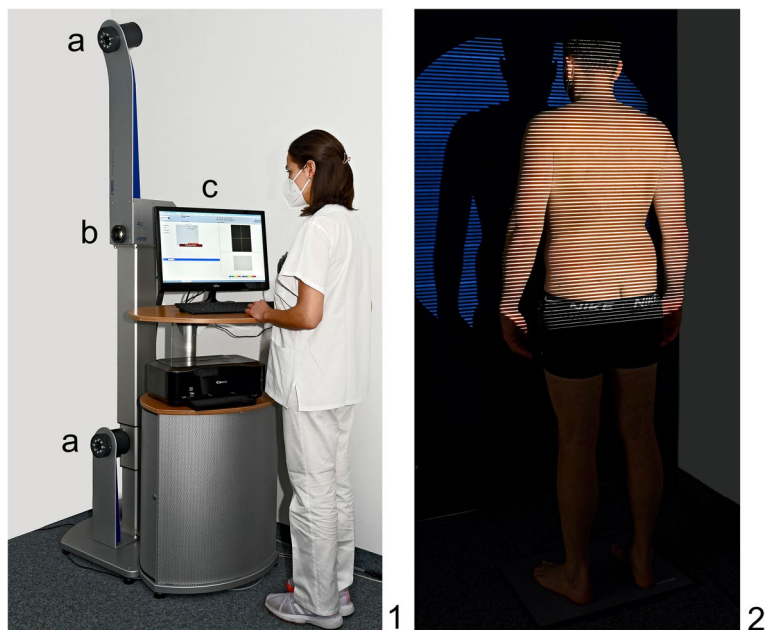
Fig. 1 Diers Formetric 4D equipment: (a) Camera units for image capture. (b) Projector which generates the line grid projection. (c) Workstation incorporating the software DiCam v2.5.15 (DIERS International GmbH; Schlangenbad, Germany). The image-captured line grid
